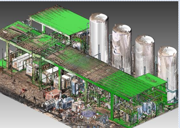
ABOVE: Point Cloud with 3D Model with AVEVA E3D
