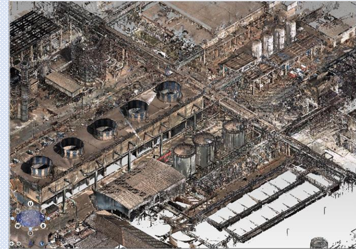
Point Cloud of a Chemical Plant Pakistan captured by 3D Engineering Surveys Ltd. in 2022
